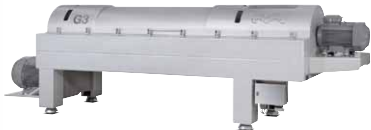
Decanters Decanter centrifuges are normally based on horizontal separation technology, which works at a speed of 5,000 revolutions per minute. They are used to separate large particles and are thus commonly used in such applications as the dewatering of sludge in wastewater treatment plants, olive oil production, distilleries and handling drilling mud in conjunction with oil extraction.
