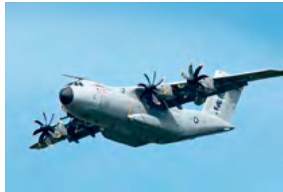
The most powerful turboprop in the Western world – the TP400-D6 engine for the Airbus A400M.
