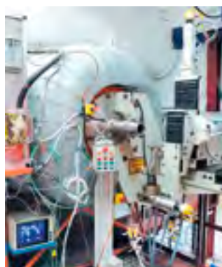
A setup used to calibrate flow sensors.
