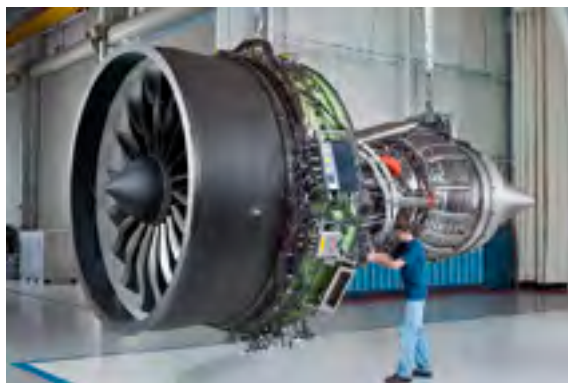
GEnx – The latest engine from GE, the powerplant for the Boeing Dreamliner, is being built in partnership with MTU.
