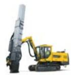
The silenced crawler rig has a noise level of approximately 10 dB(A) below that of other rigs on the market.
