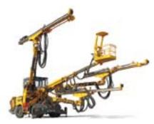
A three boom tunneling drill rig with a mechanized rod handling system for improved safety
