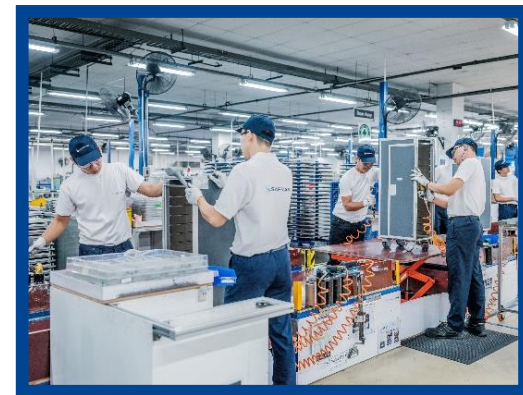
Final assembly of the trolleys
