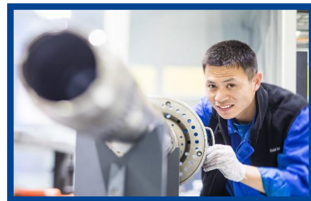
CFM56-7 MRO: Geometrical Inspection on Turbine Shaft
